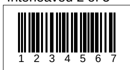
Interleaved 2 of 5 + CHECKSUM
