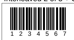
Interleaved 2 of 5 + CHECKSUM
